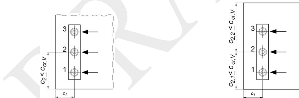
(a) ANCHOR CHANNEL CLOSE TO CORNER
