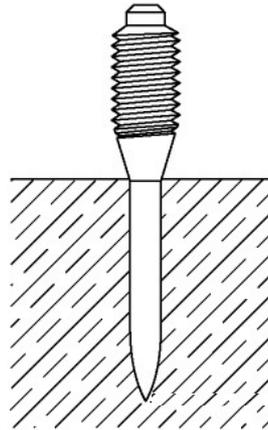
*Figure 2: Power actuated threaded stud*
