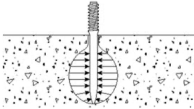
*Figure 3: PAF working principle*
