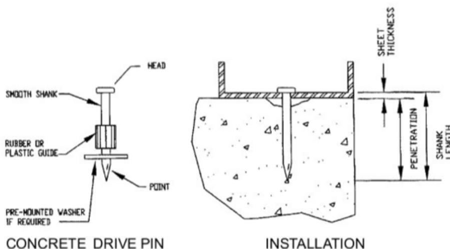
Figure 1: Power actuated drive pin connecting steel fixture to concrete
