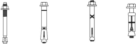
Through-bolt   Thick-walled sleeve   Thin-walled sleeve   Shield-type
