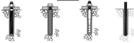
Threaded rod   Internal thread   Torque-controlled   Rebar
