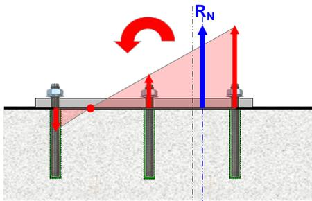
Center of anchors in tension →
