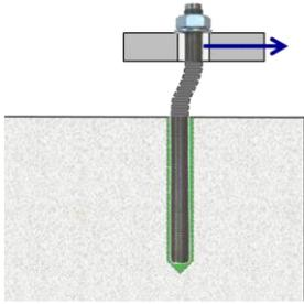
$$V_{Rd,sm} = \frac{V_{Rk,sm}}{\gamma_{Ms}}$$
