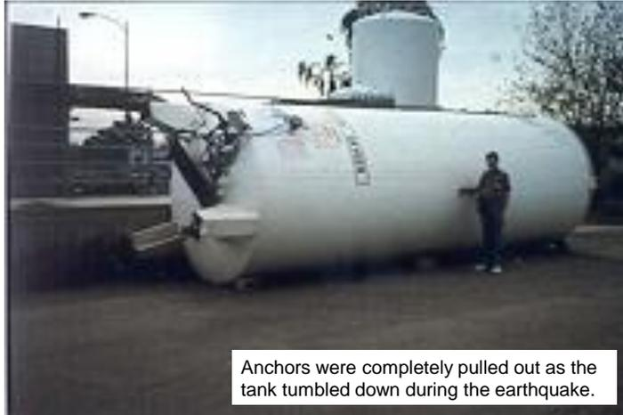
Anchors were completely pulled out as the tank tumbled down during the earthquake.
