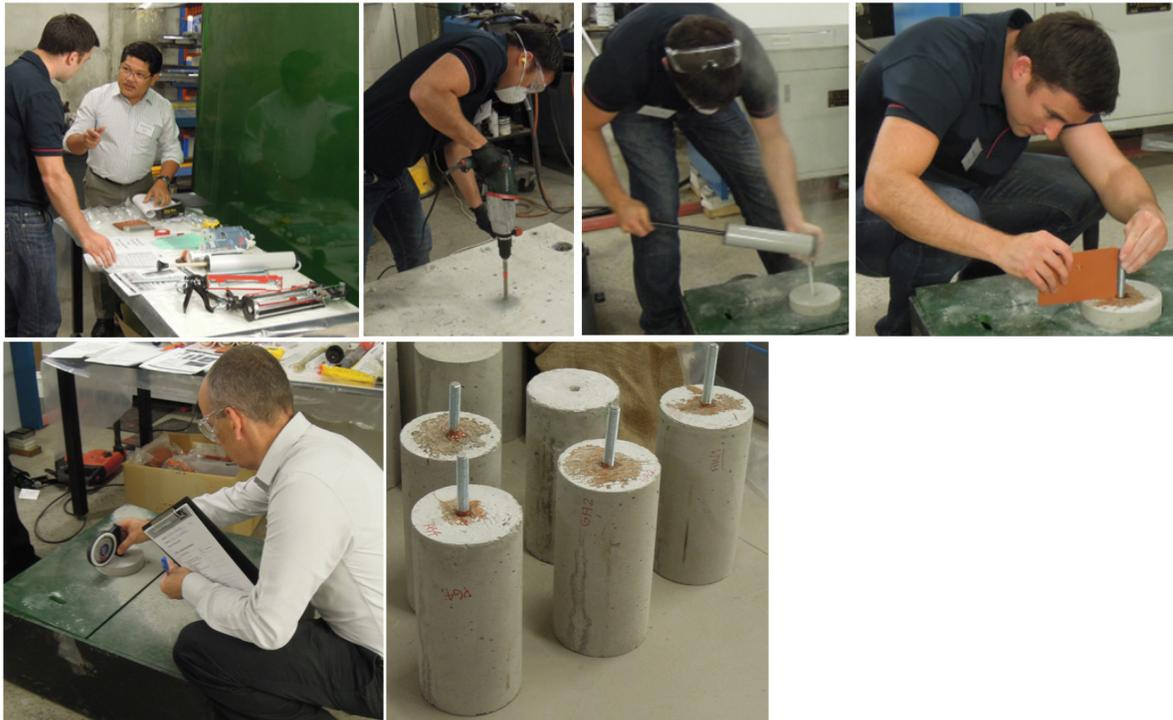
Figure 2: Vertical down bonded anchor installation
